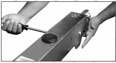
While pressing the E-stop release, pump the master cylinder with your right hand 4 to 5 times.
