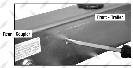
Bleeding access hole is located on the drivers side in the middle of the Actuator
